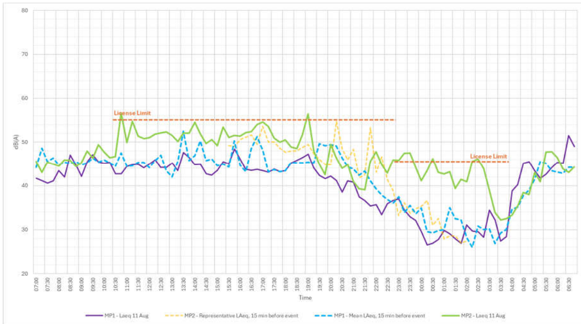
Figure 10: Comparison plot of overall L_{Aeq} at MP1 as the average of all days with no music with the Sunday 11 th when Boomtown was underway at both MP1 and MP2. Some possible exceedances against the noise limits shown at night at MP2.
